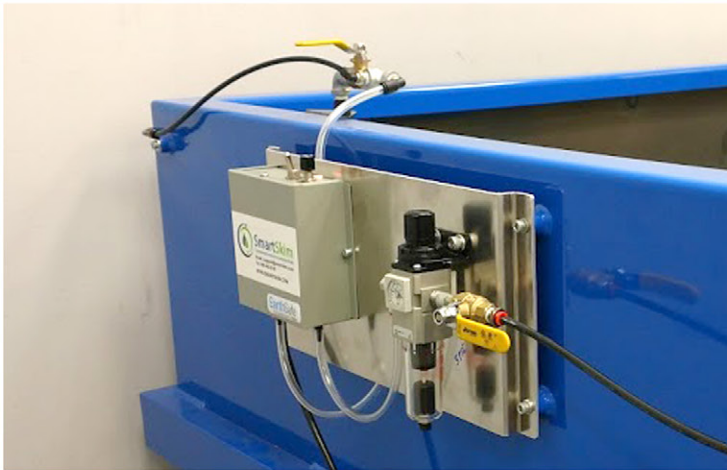
Ozone Generator on SmartSkim coolant recycling system
