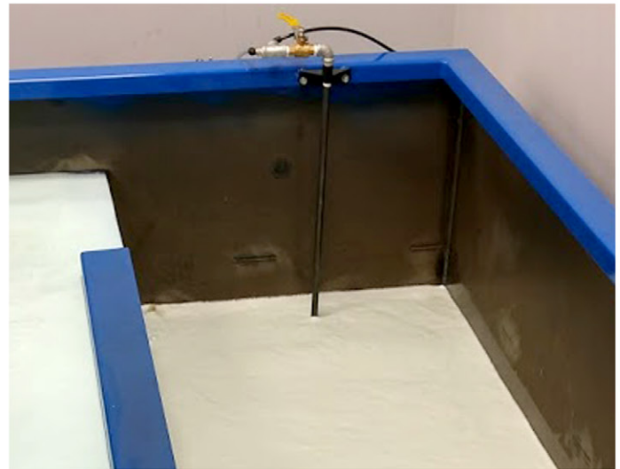
Ozone injected into coolant via dispersion tube
